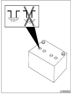
Check the fluid level in each cell. If it is necessary to add fluid, add only distilled water to bring the level up to the bottom of the filler opening. **Do not overfill.** Reinstall the vent caps.
